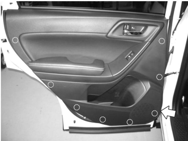
Separate the clips from the door frame at locations shown. It is easier to separate the clips if the removal is performed from the arrow section.
