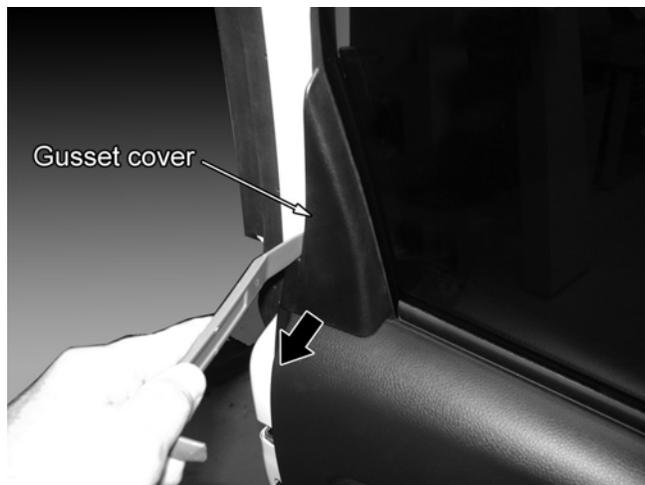
For the rear door, begin by removing the gusset cover using a plastic trim removal tool.
