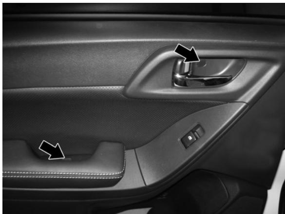
Use a small flat tip screwdriver to open the screw covers indicated.
