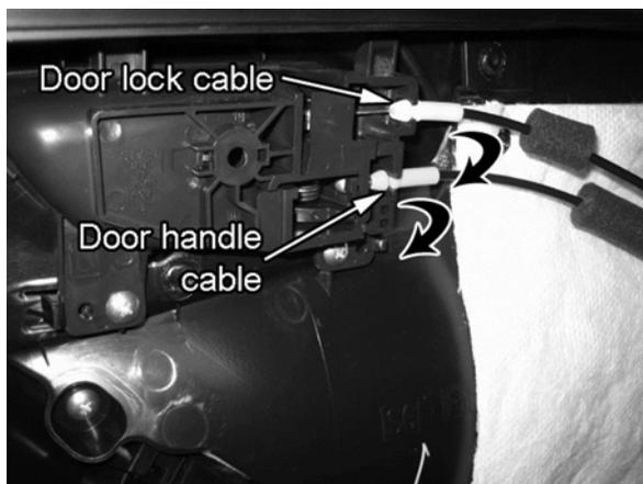
On back side of door panel, unclip door lock and door handle cables and remove.
