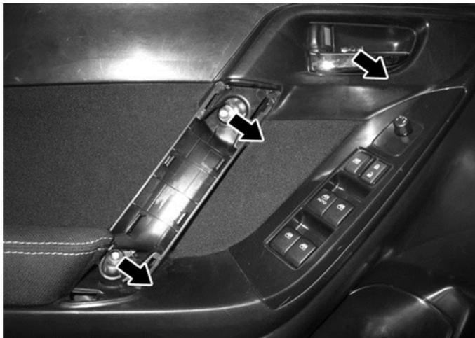
Using a Phillips screwdriver remove three screws from locations shown.
